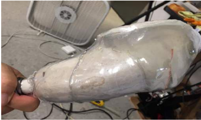
Figure 7: SSOS socket made from thermoformed soda bottle and hot glue elbow cap
