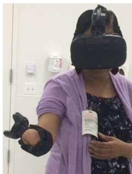
Figure 1: Subject with a transradial amputation wearing the headset and the arm tracker mounted to a custom six channel EMG cuff to control the virtual arm using pattern recognition control.
