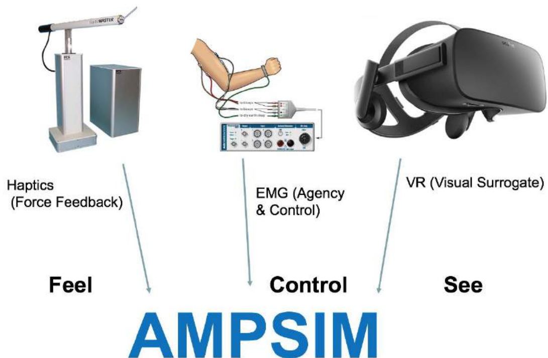
Fig. 1 The three elements used by the AMPSIM system for Phantom Limb Pain treatment
